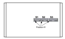
When shipped from the factory, the modem is set for the most commonly used configurations (Default configuration: <u>Only S3 position 9 is closed</u>). All other positions are open:
