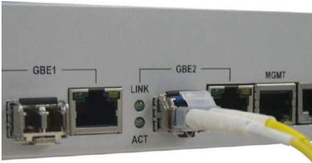
Figure 1-13 Connecting optical fiber to the trunk port
