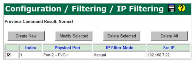
5224AV-2GBE/2SFP supports 20 allowed IPs per bridge port, ten static (manually configured) and ten dynamic rules.
