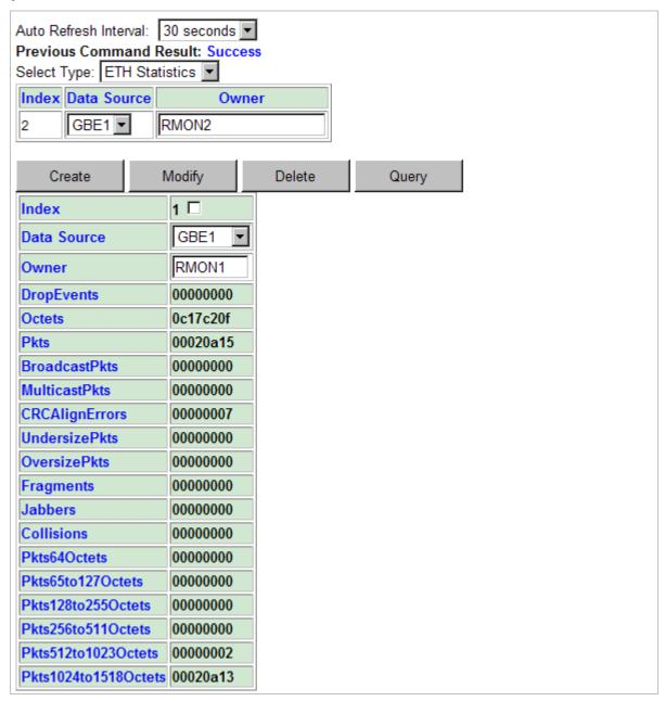
This option is for displaying the Ethernet interface RMON data. Click on the Data Source drop-down list and select GBE1 or GBE2. Type in an owner name and then click on Create button to create a new ETH statistics entry. An owner is the entity that configured this entry and is therefore using the resources assigned to it.
